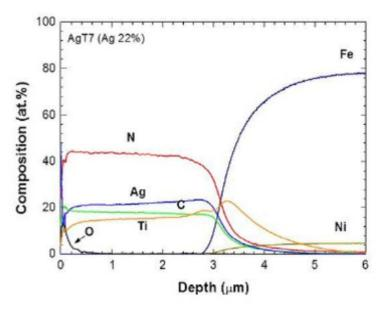
GD depth profile of a coating deposited by magnetron sputtering
