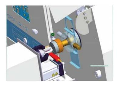
Schematic view of the LI bell mounted on the GD Profiler 2 Instrument
