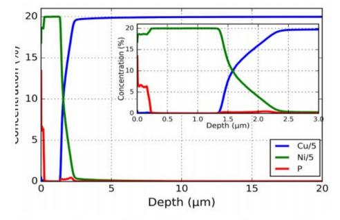
Quantified elemental depth profile for the sample shown. By establishing a set of calibration curves, it has been possible to convert the relative GDOES analysis presented in a quantative result.
