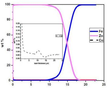
Pulsed RF GDOES depth profile (insert: the distribution in the layer)
