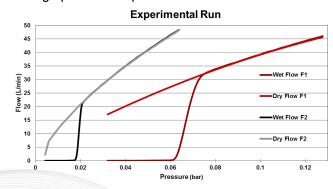
Figure 3: Measured flow rate versus pressure for the two filters F1 and F2.
