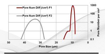
Figure 6: Differential pore number per unit area versus pore size.
