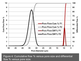
These differences are also evident when calculating the pore number per area (Figure 5) and differential pore number per area (Figure 6). It is inferred that a greater number of pores for F1 show dimensions less than ~10  $\mu$ m and material F2 has more pores in the range from 30 to 40  $\mu$ m.
