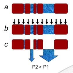
Figure 1: (a) A completely wetted sample (b) experiences a gas pressure from the upstream to the downstream which (c) forces the wetting fluid from the larger pores (P1) then to the smaller pores (P2) as the pressure increases.
