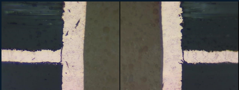
Optical microscope image showing complete layer separation in the inner conductive layers of the circuit board. Note: these images correspond to analysis done to the board itself and are not associated with a specific component.
