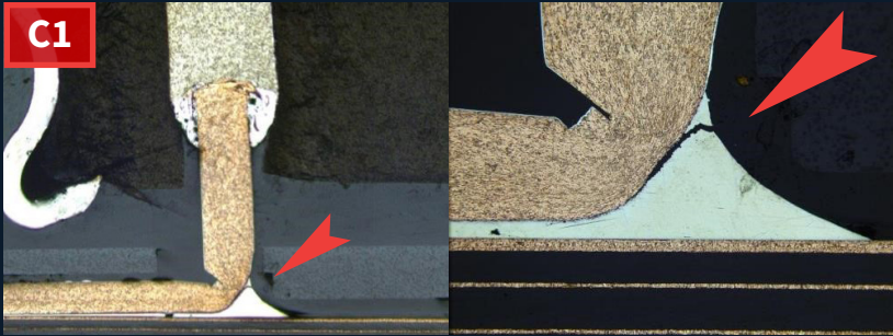
At left is an optical microscope image of the cross-sectioned segment of the C1 capacitor. The left-hand pin had a fracture through the solder connection, which is magnified in the optical image at right.
