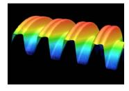
Extracted segment of 3D model generated from grooves in a screw.
