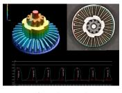
3D image of tiered gear with 2D scanned image and extracted 1D line.
