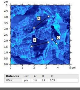
Figure 5: Grain size measurements from the phase image showing differences in the regions of different contrast.
