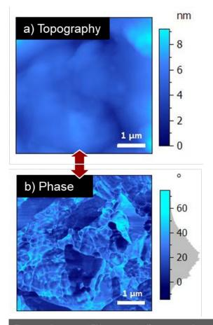
Figure 4: a)  $5x5 \mu m$  AFM topography (forward trace) image of the glove surface showing no particular differentiation in materials. b) Phase (forward trace) image of the same region showing regions of different materials, possibly the filler or pigment added to the rubber.
