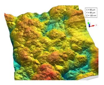
Figure 3: An 80x80  $\mu m$  3-D topography (forward trace) AFM image of the nitrile glove surface.
