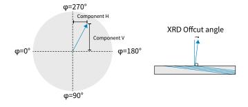
Figure 1. XRD orientation and offcut angle direction for Rigaku SmartLab measurements
