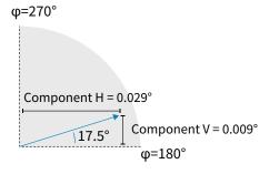
Figure 3. Measured offcut orientation and components of NIST SRM 1995  ${\rm Al_2O_3}$  wafer
