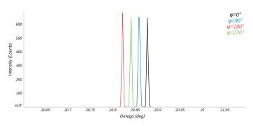
Figure 2. Overlay plot of the four Omega scans for the NIST SRM 1995  ${\rm Al_2O_3}$  wafer
