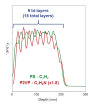
A depth profile of a poly(styrene)/poly(2-vinyl pyridine) (PS/P2VP) copolymer blend approximately 200 nm-thick on a Si substrate. The profiles and 3D image data expose the 3-dimensional structure and composition.
