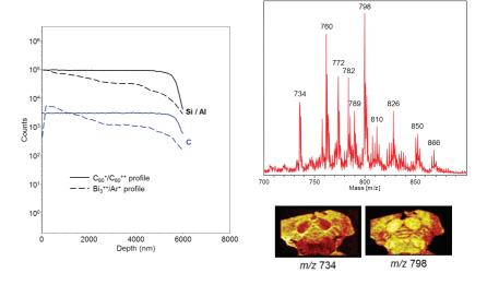
(LEFT) Depth profiles of a 6  $\mu$ m-thick aluminosilicate sol-gel on copper by Ar and  $C_{60}$  sputtering. The  $C_{60}$  ion beam does not produce the differential sputtering artifacts produced by the Ar ion beam. Additionally, the  $C_{60}$  analysis beam does not produce the surface transient artifact that is produced by the Bi analysis beam.
