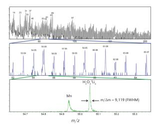
A TOF-SIMS image, collected in 5 minutes using the HR² mode of analysis, of a FIB-sectioned lithium ion battery anode showing the distribution of  $C_6H_{11}O^+$  (m/z 99) and  $C_7H_{15}O^+$  (m/z 115) ions. The lateral resolution was measured to be  $\leq$  150 nm in both ion polarities. The spectra demonstrate excellent signal-to-background and high mass resolution for full chemical and isotopic characterization.
