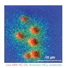
The power and utility of  $HR^2$  mode imaging is exemplified in the surface analysis of micro droplets. In only a 6 minute acquisition the micron-sized droplets are spatially resolved, and the high mass resolution spectrum allows molecular identification.
