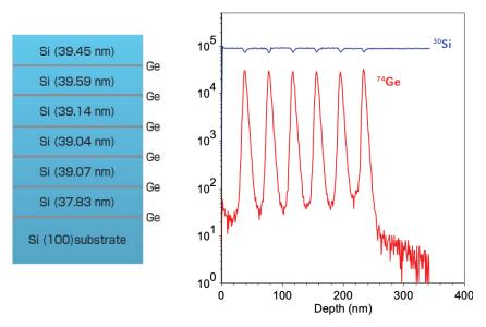
A depth profile of a multi delta layer (MDL) sample of Ge in Si was acquired using a 30 keV Bi<sup>+</sup> primary ion beam (50  $\mu$ m square raster) and a 1 keV Cs<sup>+</sup> sputter ion beam (200  $\mu$ m square raster). The Ge delta layers are 0.4 nm thick.
