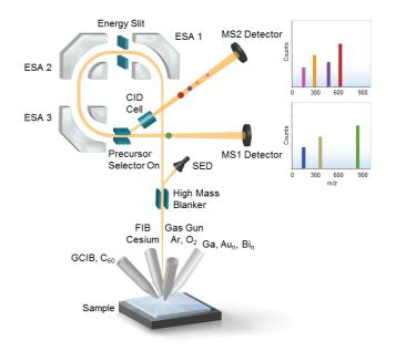
The schematic highlights the triple electrostatic analyzer (ESA) design of the *nanoTOF* II's Parallel Imaging MS/MS spectrometer. Selected precursor ions are deflected at keV energy into a collision-induced dissociation (CID) cell for fragmentation. The product ions are collected at the MS2 detector. Any ions not within the monoisotopic precursor selection window continue on their original flight path to the MS1 detector.
