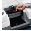
close off manual purge ports. Smart Purge senses when you are changing samples and automatically turns up the purge. This ensures rapid recovery of purge - in a few seconds!
