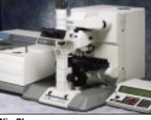
Nic-Plan Introduced remote sample aperturing with grazing angle and ATR objective
